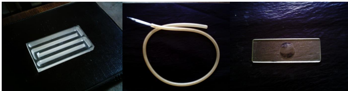
Fig. 4 Bogorov tray, micropipette equipped with rubber hose with a mouthpiece and slide with cavity
