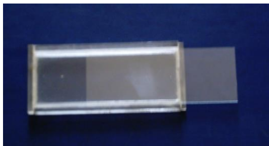
Fig. 3 “Pencil box” chamber for enumeration of ciliatoplankton.
