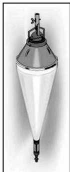
Fig. 1 Small Planktonic net Apstein Hydro-Bios (55 \mu\text{m} mesh size nylon)
