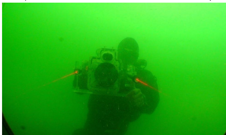
Fig.2. Underwater camera with the laser pointers
