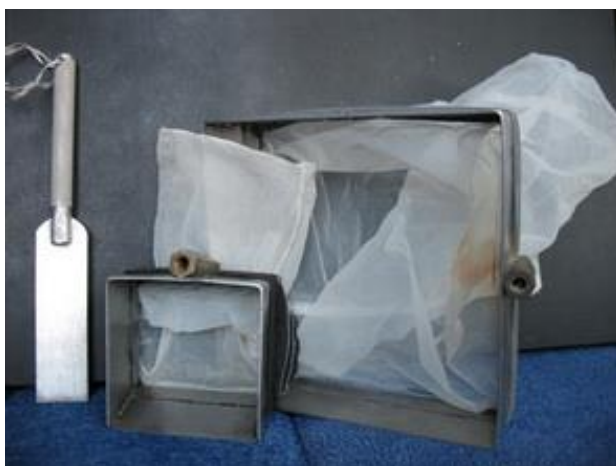
Fig.1. Scraper and periphyton frames for the quantitative samples of macrophytobenthos
