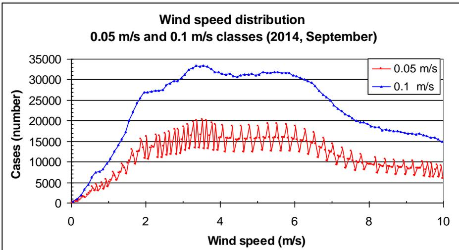
Fig. 15. Wind speed distribution of the same subset at different width classes
