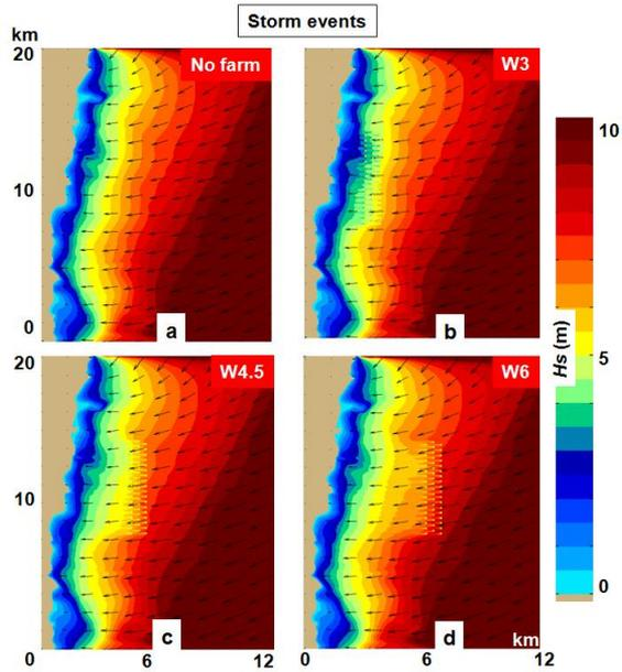
Fig. 6. The expected impact of the wind farm on the wave fields reported during a storm event, where: a) no farm; b) W3 scenario; c) W4.5 scenario and d) W6 scenario
