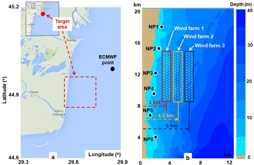
**Fig. 1. Definition of the target area and set-up, where: a) overview of the target area; b) SWAN computational domain where can be observed the three case studies taken into account and also the locations of the reference points NP1-NP6**
