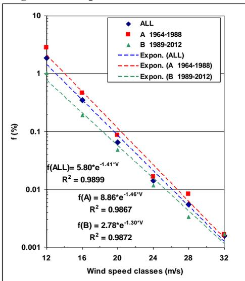
Fig. 6. Wind speed distribution - MA
