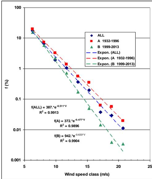
Fig. 2. Wind speed distribution - OD
