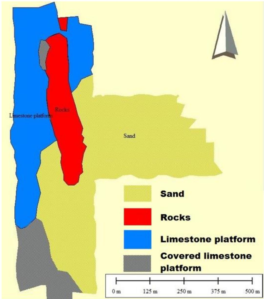
Fig. 8. Acoustic seabed classification of the study area
