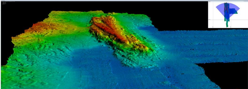
**Fig. 7. Perspective view of the bathymetry grid. The upper right corner - positioning of the perspective view over the survey area**
