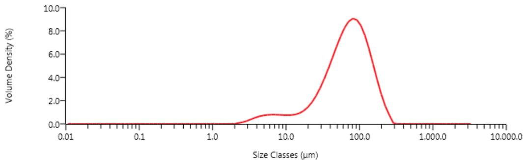
**Fig. 6. Grain size histogram of a sediment sample form seabed type 3**
