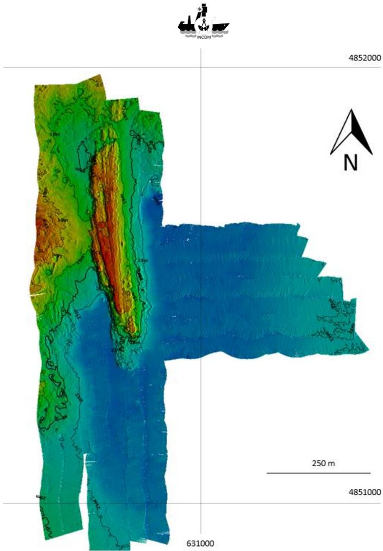
Fig. 3. Bathymetry map of the surveyed area. Coordinates UTM, zone 35 N, WGS84 ellipsoid
