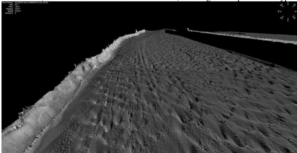
**Fig. 2. 3D visualization of interferometric sonar measurements; side-scan mosaic overlapped on bathymetry - Danube river, near Corabia, Romania**
