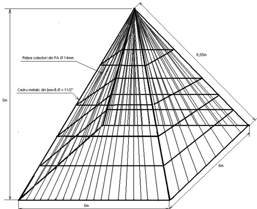
**Fig. 4 - Submerged pyramid-shaped structure**
