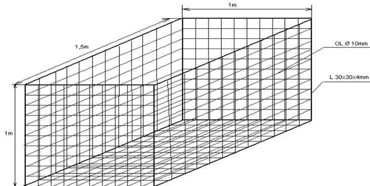
**Fig. 3 - Metal frame for gabions**
