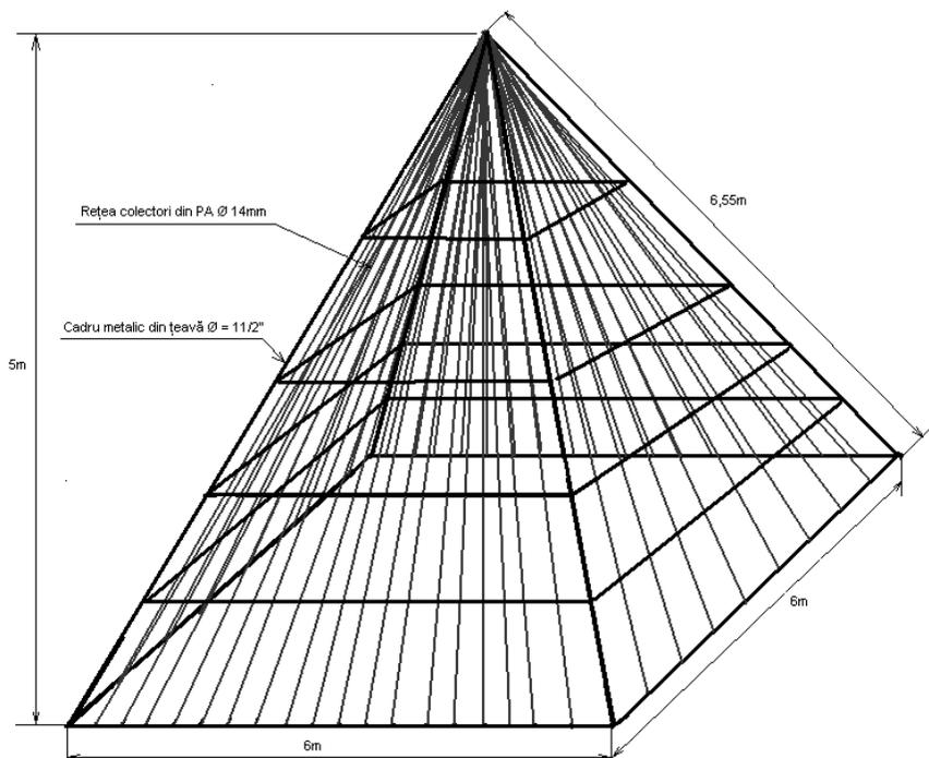
**Fig. 4 - Submerged pyramid-shaped structure**
