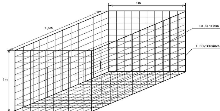
**Fig. 3 - Metal frame for gabions**
