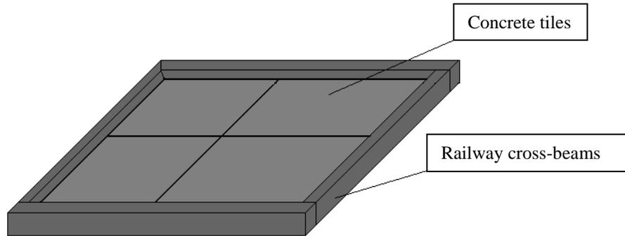
**Fig. 2 - Concrete tile platforms**
