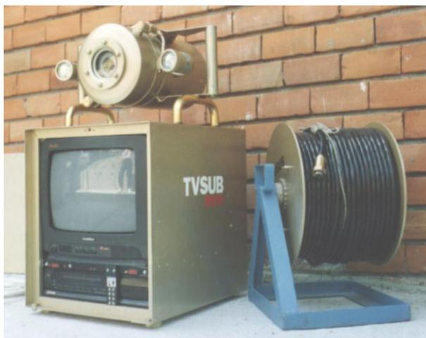
Photo 3 – Installation tv sub *ITS Ciclop*
