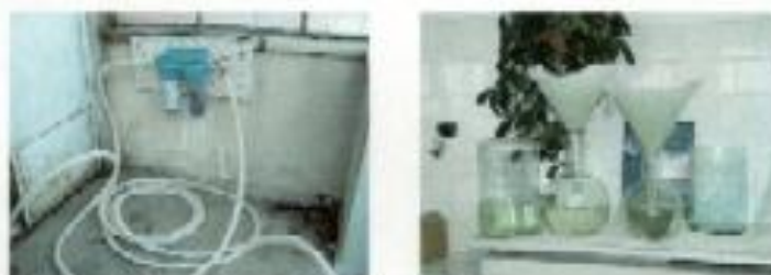
Fig.4 LABORATORY INSTALATION FOR FILTRATION AND ADDITION OF MARINE WATER
