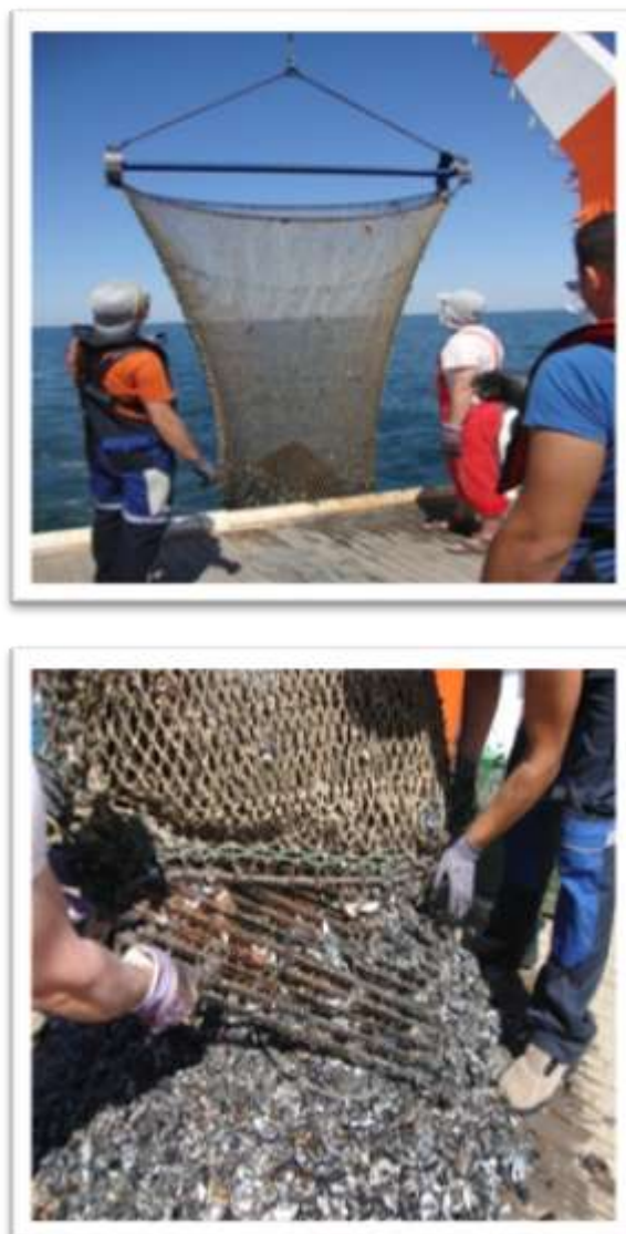
Figure 10: Beam trawl for sampling marine litter
