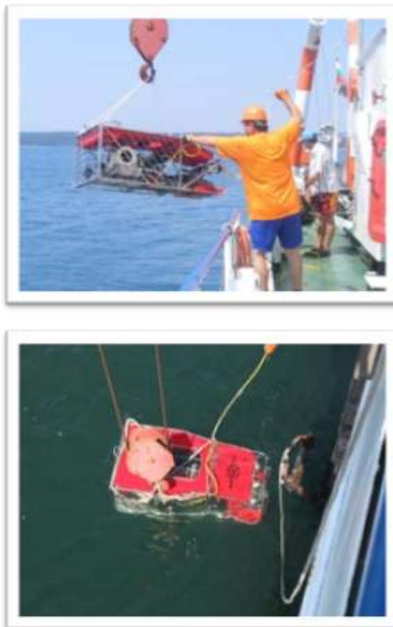
Figure 11: Remotely Operated Vehicles (ROV) Mariscope
