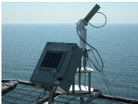
Radiometru oceanic instalat la Platforma "Sectia 7"
